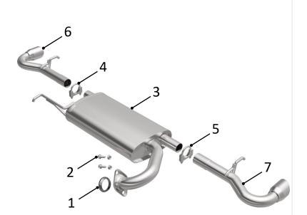
(Carefully read all instructions before installation) Disconnect the vehicle's battery before removal of the OEM exhaust system. This will prevent electrical accidents and will reset the computer if it applies to the vehicle. Remove existing exhaust system from the vehicle. Only remove parts that will be replaced. Clean existing flange with a wire brush to ensure proper sealing.
